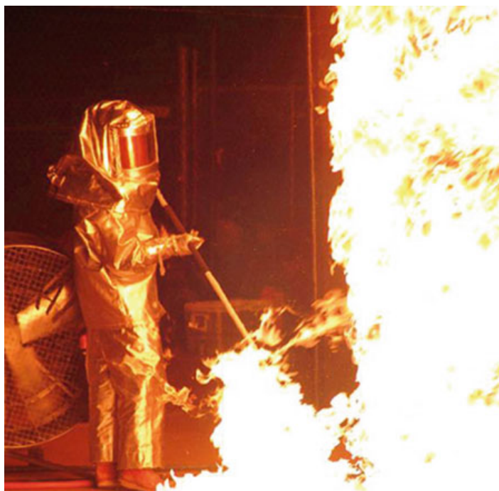
Fig. 6.10 A “fire entry suit” designed to spend short moments in contact with fires up to 1,000 degrees Celsius. Image credit: Meikangco.com
